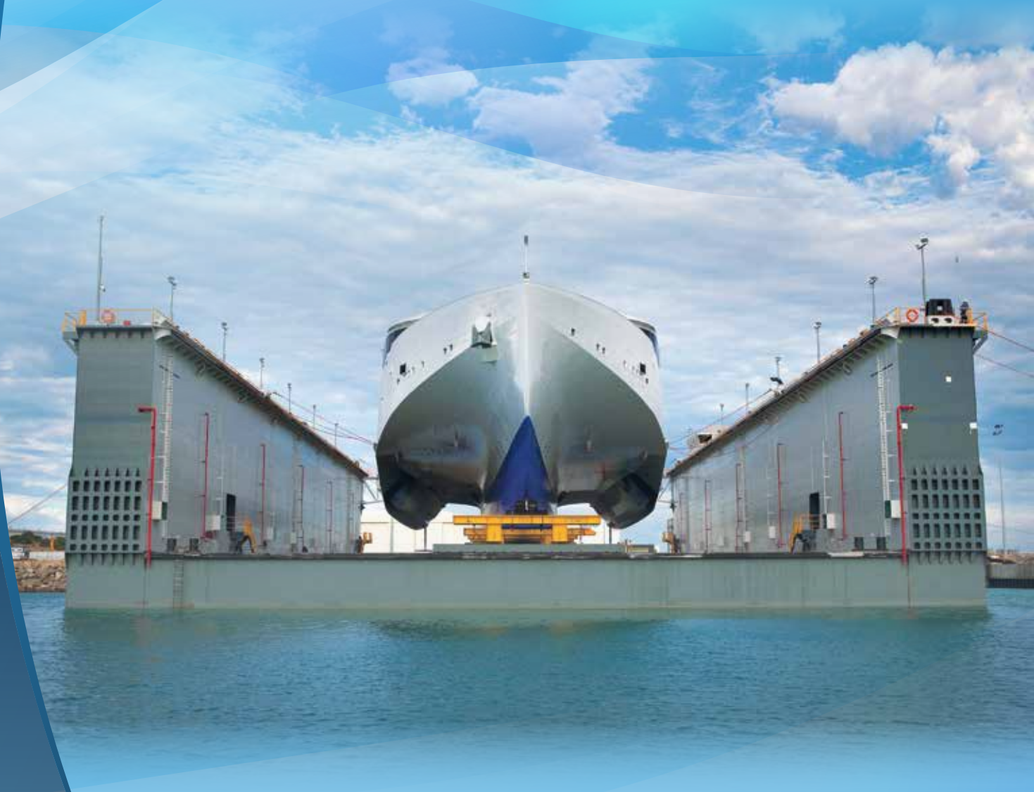
▲ NEXT GENERATION 102 TRIMARAN IN DRY DOCK
